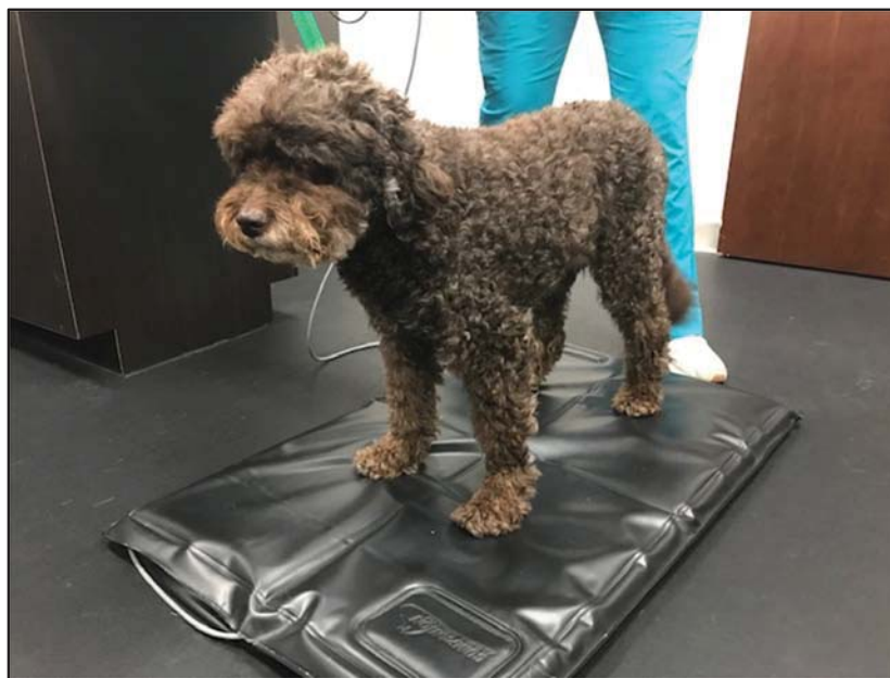
Figure 1: Picture of a dog standing on the computerized stance analyzer mat. The percentage of a patient’s body weight placed on each limb while standing on the mat is analyzed with normal weight distribution for each front limb 30% and hind limb 20%.
